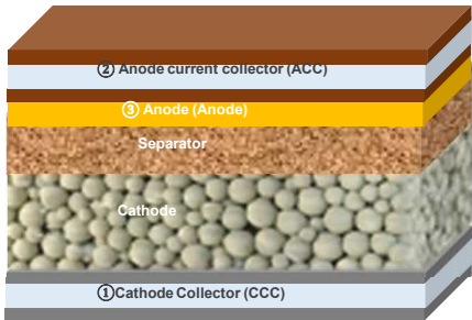
Lithium battery structure with double-sided deposition film
