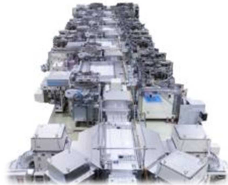
ZELDA Series: Vacuum evaporation equipment for OLED production
