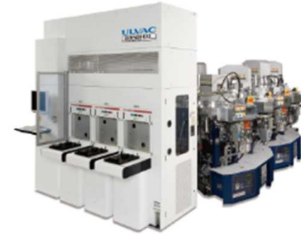
ENTRON-EX: Sputtering systems for semiconductor production
