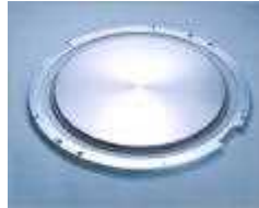
Target used in sputtering
