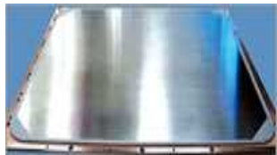
Target used in sputtering
