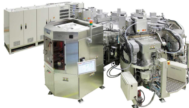
PZT-MEMS production equipment
