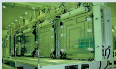
Plasma CVD system for photovoltaic cells
