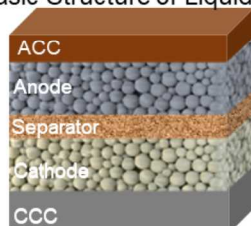
Basic Structure of Liquid LiB
