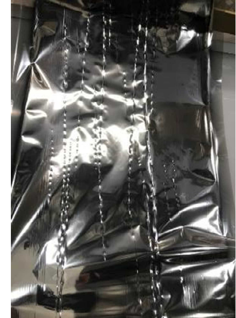
Wrinkles and tears. Thermal damage occurs
